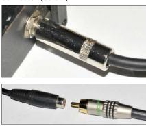
RCA type male and female connectors (above) transport line-level signals from CD players, MP3 players or other audio sources. They, too, only work in female, through a corrupted physical a male/female arrangement.
